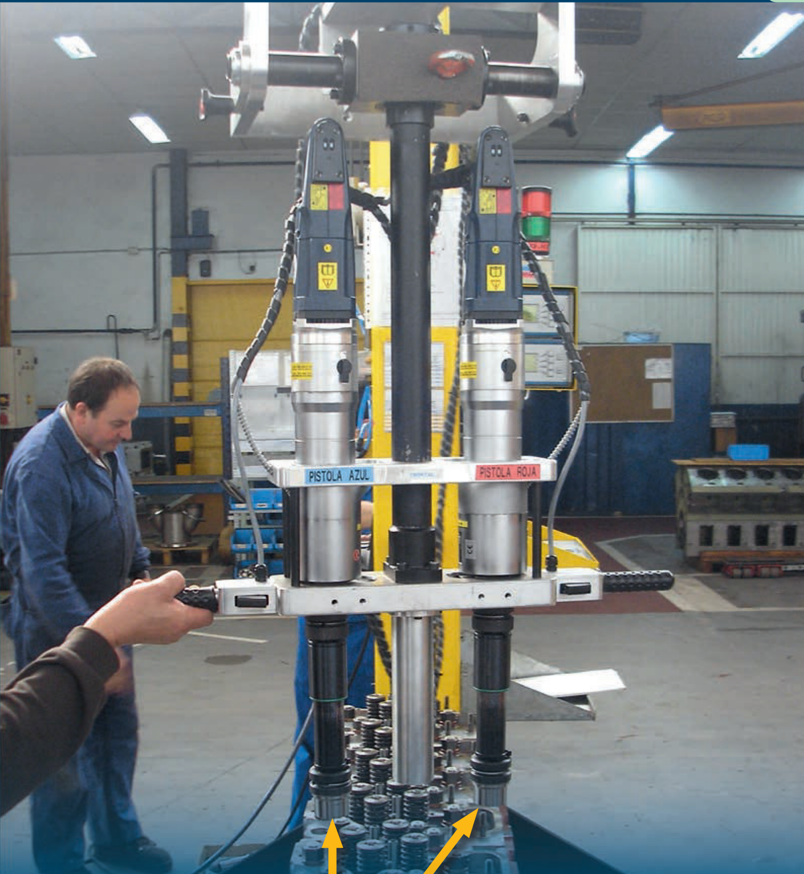
DE Double nutrunner for production line cylinder head assembly
